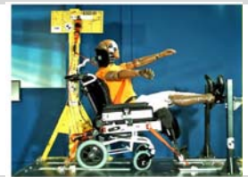
CRASH TEST Model B30 and B60 are suitable to be transported in a vehicle according to ISO 7176/19 and ANSI RESNA WC/19 standards.
